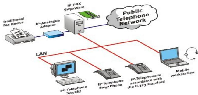
A **PBX** is a telephone switching system that provides communication between a number of phones and trunk lines for departments within the company. A typical business PBX includes external and internal phone lines, computer servers that manages the calls and manual consoles.
